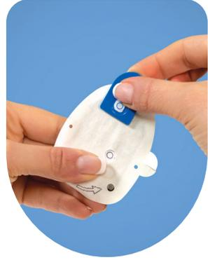
3. Remove the Pod's needle cap
