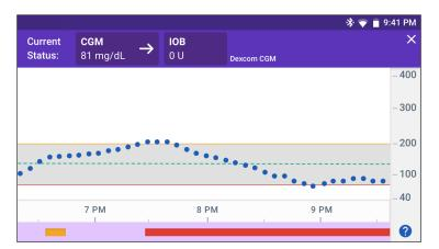
When the Omnipod 5 System is in Automated Mode: Limited state, the graph heading is dark gray.
