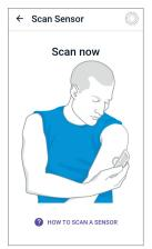
Place the back of your Controller up to the Sensor and scan it. The lower third of the Controller should almost touch the Sensor.
